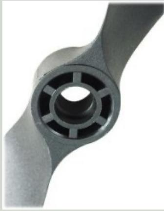
Hub balancing is done by carefully drilling very small holes (say 2mm diameter) on the lighter side of the back of the hub, and filling the holes with a liquid ballast material or small pieces of lead, or perhaps fishing shot, sealed in. Obviously the lighter side will be identified when using your prop balancer.
