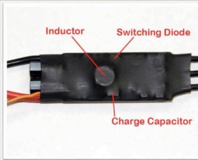
The nice thing about the Switching BEC is that it puts or full current, regardless of the input voltage. This is much better than the Linear type
