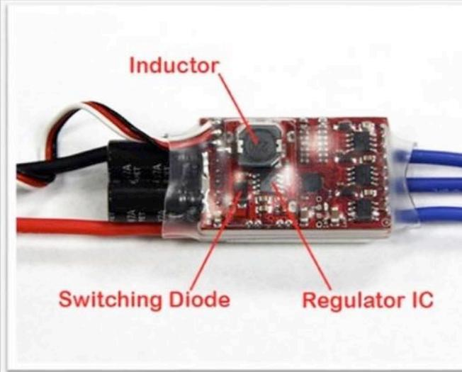
On a speed controller with black heat shrink, the switching type ESC can be identified by the large inductor, with is about 1/2" or 12mm square, as seen in the next photo.
