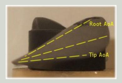
The picture above approximately illustrates how the Angle of Attack varies along the blade length.
