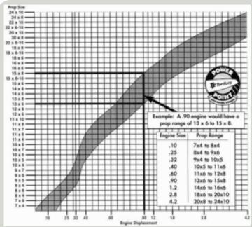
speeds and loads. As with IC, electric motor manufacturers give a specific propeller size range for their motors but it's more critical that the range must be adhered to. Over-propping can do irreversible damage to electric motors and ESCs, because an incorrect propeller will force the motor to work harder than it was designed to.
