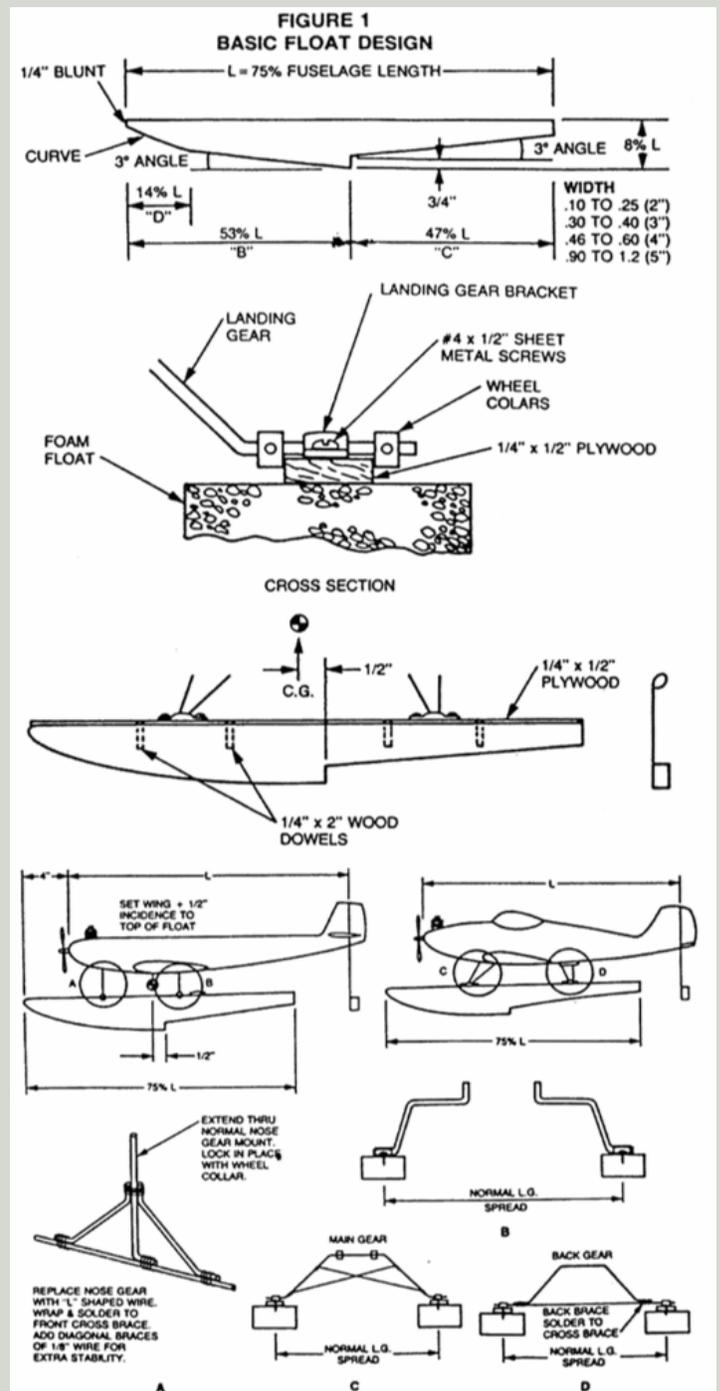
actually a factor of the overall weight that the floats have to support, so use the table in Figure 1. For our example we will use a width of 4". The nose and tail up-sweep angles are as low as you should go. Increasing the aft sweep from 3° to 5° will allow the aircraft to break the water suction easier but also the aft end of the aircraft may ride lower in the water. I have used both angles and think that in the future I'm going to stick with about 4°.
