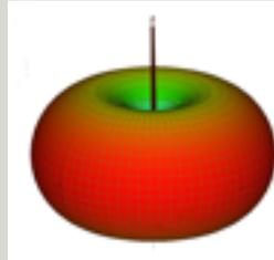
transmitting antenna itself. The image on the left graphically illustrates the radiation pattern of ANY standard ¼ wavelength "whip" antenna. It actually looks similar to a donut and may best be imag-
